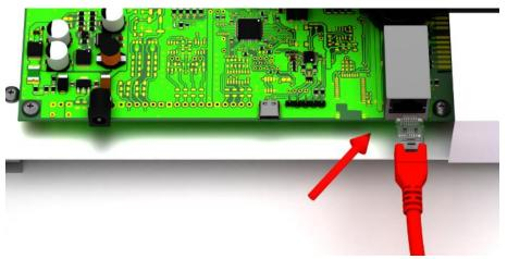
Displays with Ethernet interface are connected with an Ethernet cable cat. 5 or higher. Modern PCs or laptops recognize the cable type automatically.
