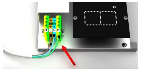
The unit has a metal housing. It corresponds with protection type I and needs a protective conductor connection. The connecting cable for the power supply must contain a protective ground wire connection with sufficient cross-section (DIN VDE 0106 Teil 1, DIN VDE 0411 part 1).
