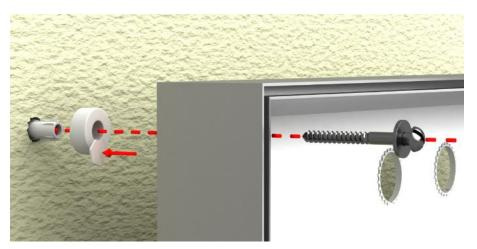
The cables can then be fed between wall and device (surface mounting). To fix the spacers during installation use the included hexagonal self-adhesive stripes.
