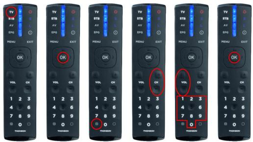
During input, the internal channel number of the corresponding field can be displays by pressing the button INF. This is indicated by a left-aligned digit with varying brightness. By pressing the info button INF again, the display changes back to input mode.
