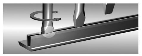
Insert the front pane and the connectors. Spread the connectors slightly with a screwdriver before inserting so that they are stuck firmly in the housing frame. Check that the connectors are fixed so tightly after insertion that they can not be removed without tools (lever tools).
